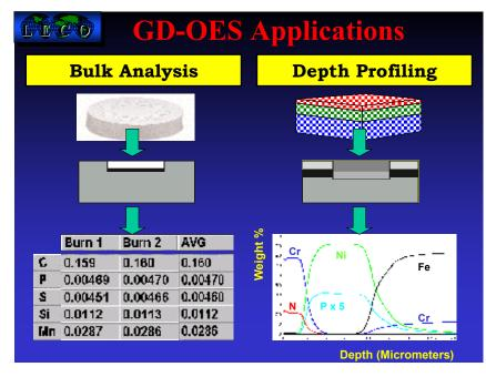
**Bulk analysis** can provide the elemental composition of the sample in less than one minute.
