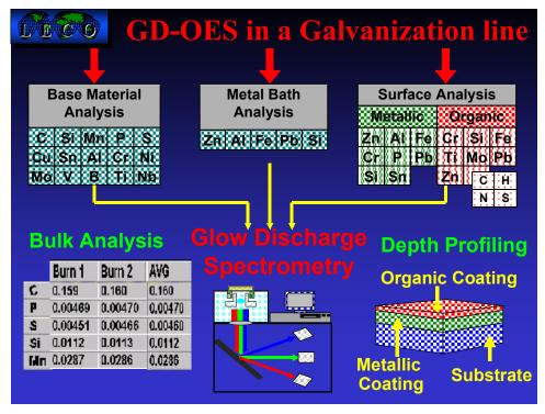
The figure to the left shows where the Glow Discharge technique can be used in a Galvanization line.
