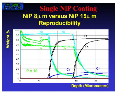
These profiles confirm the expected thickness of the NiP coatings (8 and 15 micrometers). The 15 micron NiP coating shows a perfect reproducibility in terms of thickness and composition. The 8 micron NiP coating shows a perfect reproducibility in terms of thickness and composition for the Ni, but we can note that the phosphorus concentrations are not the same. Additionally, the P profile is not constant and shows a non-homogeneity.
