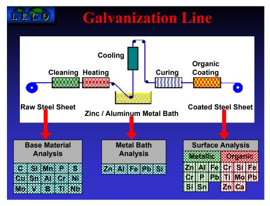
Schematic of a classic galvanization line with an organic coating at the end of the process.
