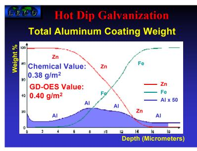
example, thickness and coating weight can be obtained immediately after the acquisition of the profiles.
