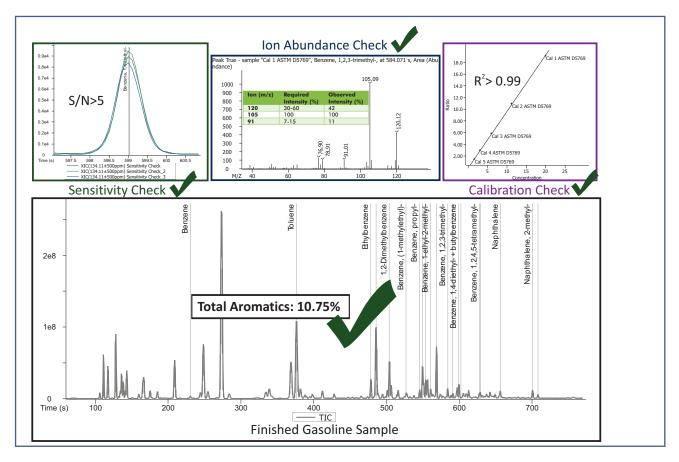
Figure 1. Total aromatics were determined for a commercially available sample of 93-octane gasoline. The chromatogram with peak markers automatically placed for calibrated analytes and deuterated internal standards is shown, along with the required method checks exceeded by the Pegasus BT.
