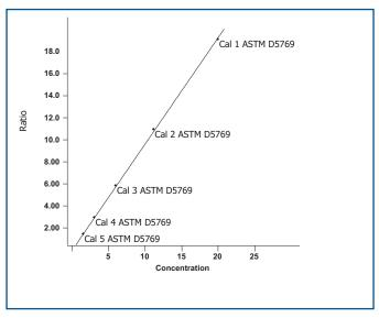
Figure 4. Linear calibration curve generated for toluene, with  $\mathbb{R}^2$  value of 0.9998.
