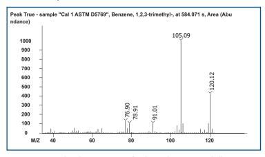
Figure 3. Deconvoluted mass spectrum for the peak 1,2,3-Trimethylbenzene at 3 mass % level.
